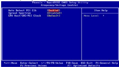
**NOTE:** This "Frequency/Voltage Control" option controls the CPU Host and PCI frequency, this page is developed by CPU and Chipset independent, some items will show up when you install a processor which supports this function.
